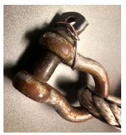
**Note: YOU** are expected to install your own pennants and **MUST** use a corrosion-resistant wire for securing your shackle pin. You are also responsible for checking and maintaining all shackles above the mooring, including their pin securement systems. **DO NOT**, under any circumstances, remove the shackle that OUW provides atop the mooring.
